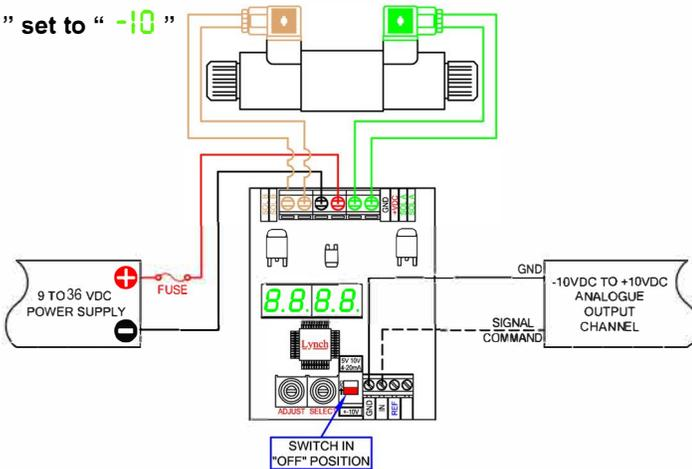
**PLEASE NOTE:** For “0 to 5 VDC” & “0 to 10 VDC” command input drivers, it is recommended to use independent negative conductors for power supply and analogue output channel (PLC/PC) to maintain command signal accuracy due to voltage drop on long cable runs.
