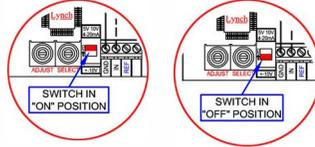
\*\*\*Applying improper Input Signal to wrong setting on the Driver may be damaging to Driver Unit and may cause driver to fault to Error Status mode\*\*\*
